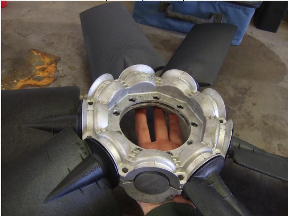
7. Place two bolts in opposite sides to squeeze the hub halves together.
