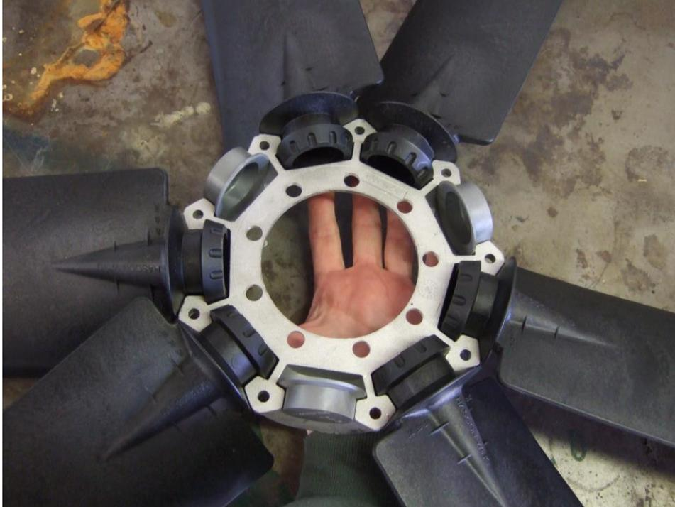
6. Place the other hub half on top of the assembly and squeeze together by hand. Be careful to keep all the pieces in place.
