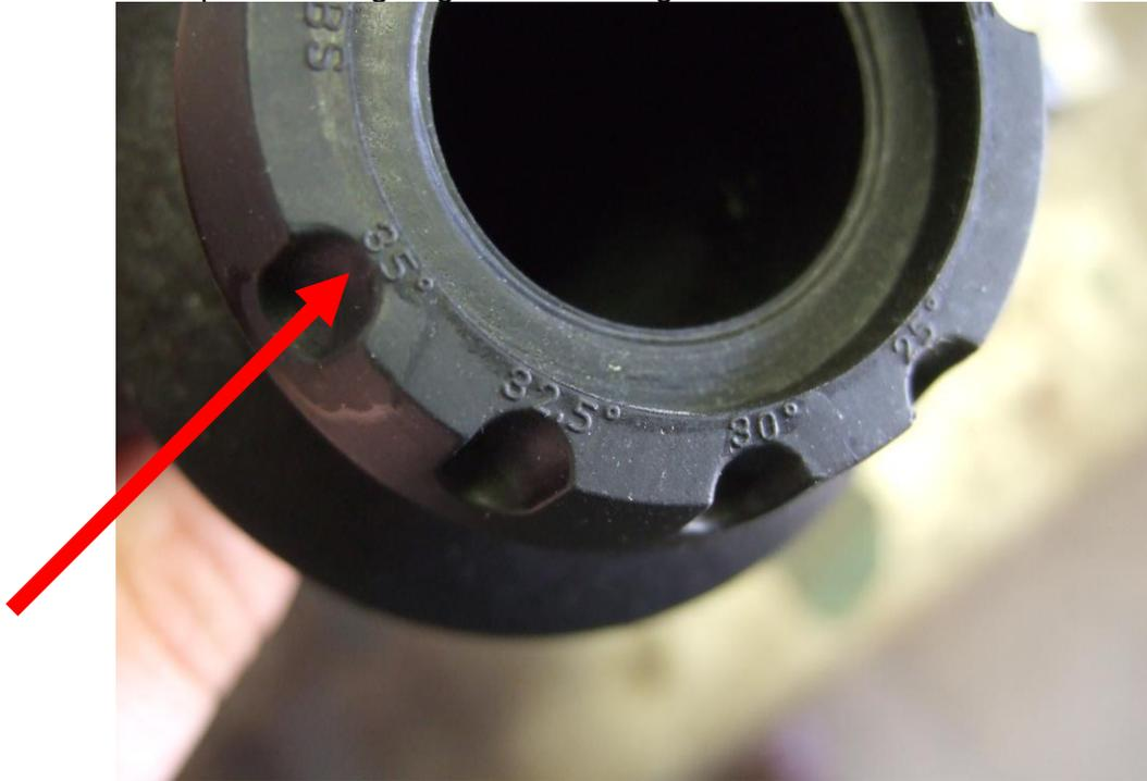
3. Place the pitching ball in the hub notch that corresponds to the blade notch you want. The 4 notches in the hub and the blade should always be aligned. Here we've chosen the 35 degree notch.
